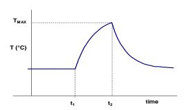
Since the "on" time is too short for the motor to reach a steady thermal condition, the load during the "on" time is permitted to exceed the continuous rating of the motor. However care must be taken so that the maximum motor temperature is not exceeded.
