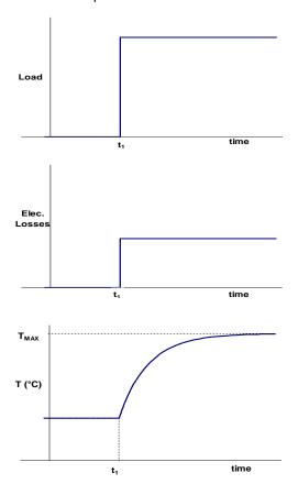
It is essential that the motor rated torque exceeds the value of load torque in order to prevent burn-out. S1 duty is used in determining the rating of an industrial servomotor. However typical servomotor duty is rarely of type S1.
