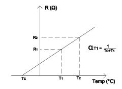
By geometry it can easily be shown that R2 = R1 [1 + aT1 (T2 - T1)] .... (1)
