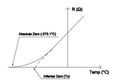
Therefore we can consider resistance as a linear function of temperature on a centigrade scale as shown below.
